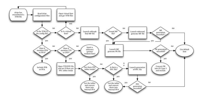
Figure 1: odvips responding to a font request in the DVI file.
