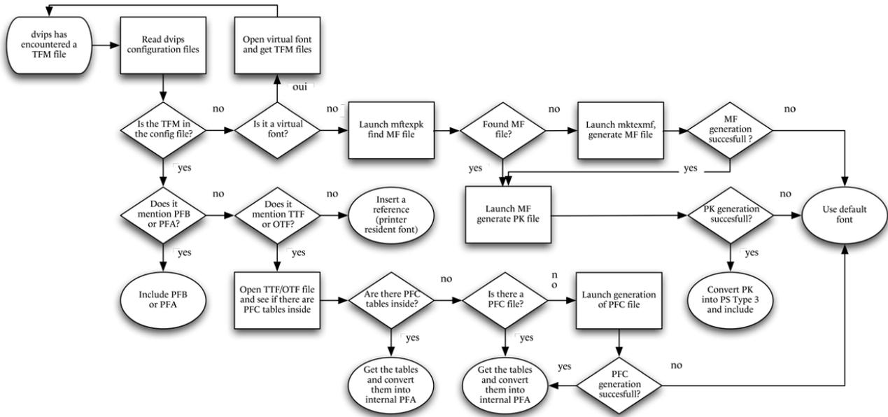
Figure 1: *odvips* responding to a font request in the DVI file.
